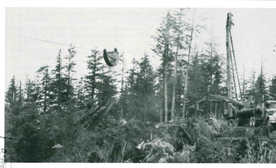
Young's new Carriage is a radio controlled unit complete with a self-energizing sealed hydraulic system. Positive in its functions it is light weight and compact in size. The unit's slack puller feature gives positive feed-out of up to 300' of dropline. Ideal for all logging operations and especially suited for selective logging.
