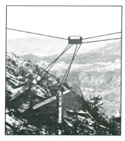
For far side logging the operator simply tightens the skyline sufficiently for gravity to run the carriage out the desired distance. The carriage is then clamped to the skyline via radio signal. The skyline is sagged to set the chokers without the carriage settling to the belly of the line. The carriage operates as a standard shotgun system when the clamp isn't used.
